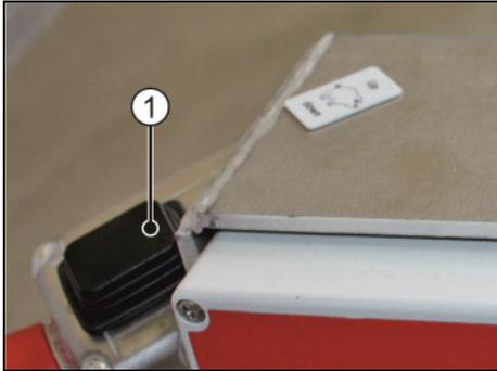
– Operate the button ROLLER DRIVE UP/DOWN and set to UP position. Keep the button in that position
