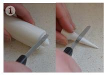
Both tips (cartridge and attachment) should be cut open far enough.
