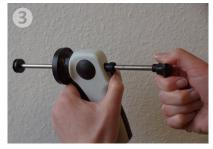
Loosen the piston rod by actuating the piston sleeve and pull it back out.
