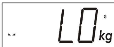
You are in the menu for setting the lower limit. LO is displayed for 2 seconds. The preset weight of 119.0 kg is then automatically displayed.
