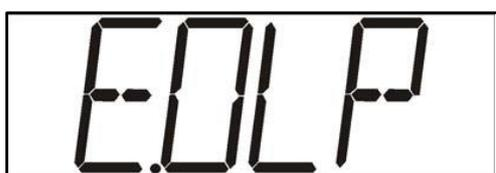
If the sample is heavier than the set weighing range, „E.O.L.P.“ (=overload) appears in the display.
