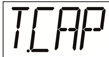
Please enter the total capacity of the cells here. Example for 4 cells with a capacity of 1000kg each. The value to be set is 4000kg.
