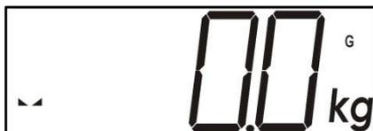
When a small amount is displayed, press
