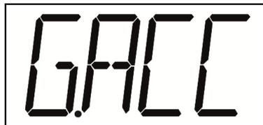
Please enter here the value of the acceleration due to gravity of the respective installation site. If you manually correct the value of the theoretical calibration with real weights at the installation site, you do not need to change this value.
